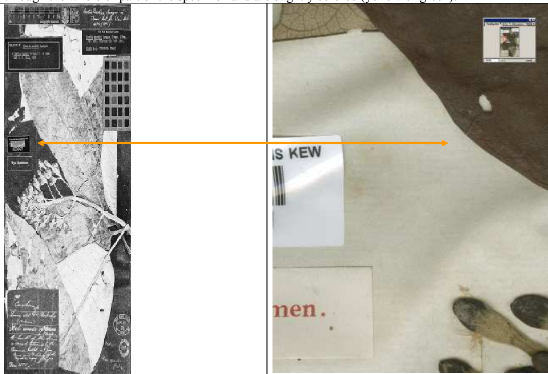
GIF image and corresponding TIF showing a vertical line due to dust in the scanner head. REJECTED IMAGE.
